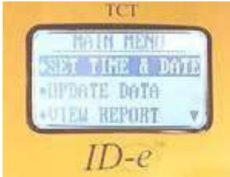
**To ERASE RECORDS...** Hold the SET button. Scroll to the erase records option on the user main menu and select with the ENTER button. Records will count down as they erase to zero or let records exceed memory and ID-e® will reset automatically to 0 records (EST about 3800 records).
